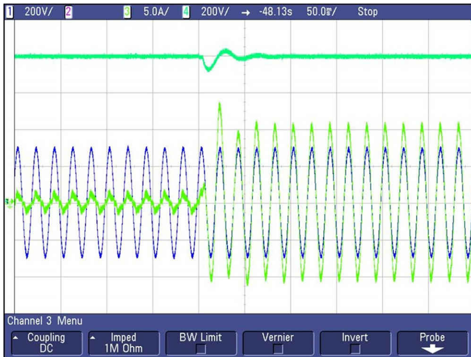
Figure 3-43. Voltage Step - 400 W → 4.4 kW
