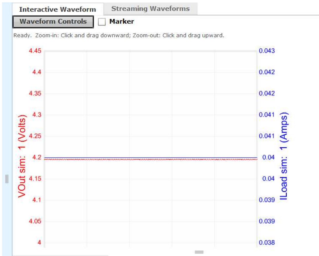
Figure 15. WEBENCH® Simulation for TPS61099 Boost Converter (Test Results)
