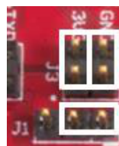
Figure 6. USB (eZ-FET) Power Jumper Configuration
