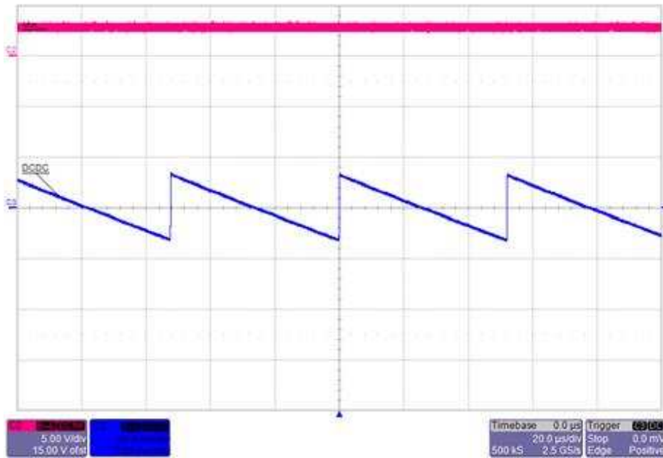
図 16. TPS62801 Output Ripple ( V_{IN} = 3\text{ V} , Load = 1 mA)
