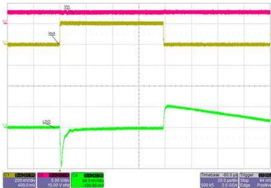
Figure 33. TPS7A10 Load Transient Response ( V_{IN} = 3\text{ V} , 1-mA to 200-mA Load Step)
