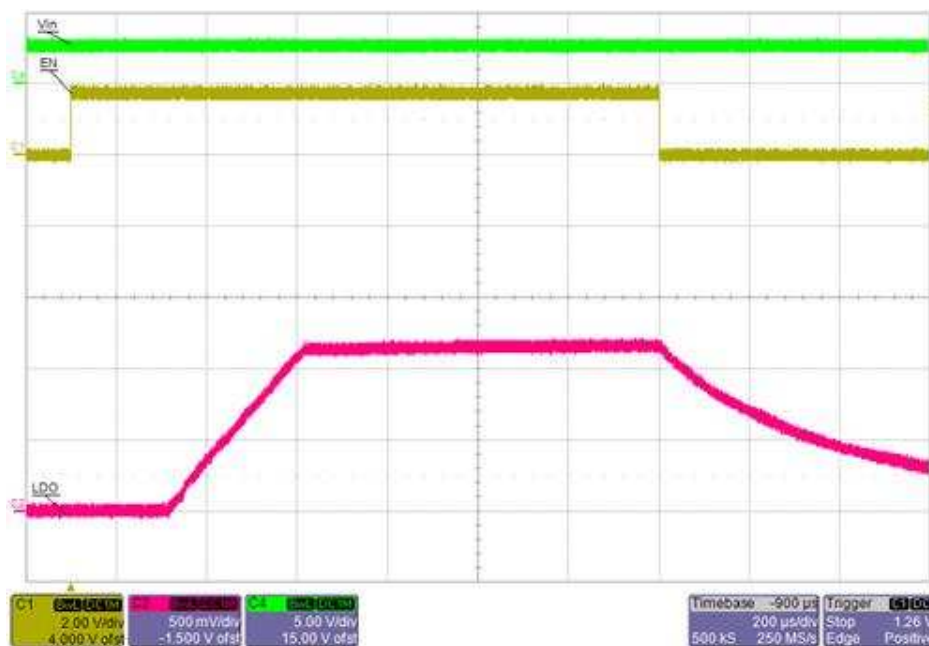
図 35. TPS7A10 Start-Up and Shutdown ( V_{IN} = 3\text{ V} , Load = 0 A)
