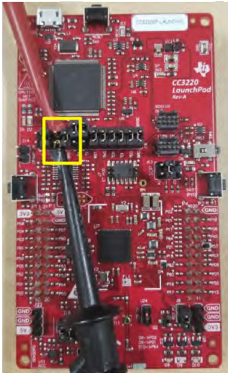
図 36. Probe Connection for Power Measurement
