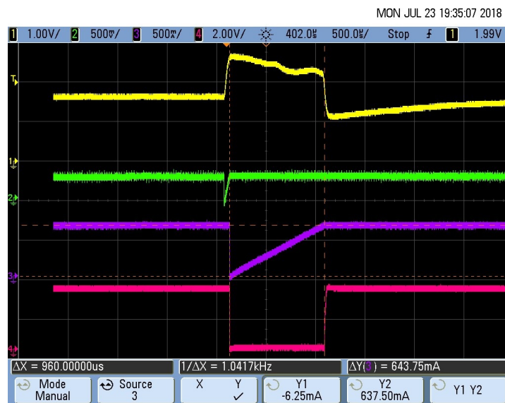
図 63. Pacemaker Detection Output (Pulse Duration T_P ) for 8-mV, 1-ms Pace Pulse
