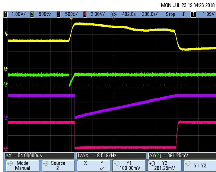
図 62. Pacemaker Detection Output (Rise Time T_R ) for 8-mV, 1-ms Pace Pulse
