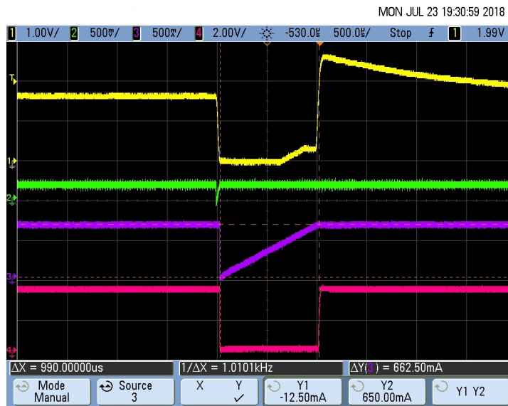
図 82. Negative Pace Signal Detection - Negative Pace Pulse Detected by setting the Polarity Check (CH-6) Output of the DAC Low
