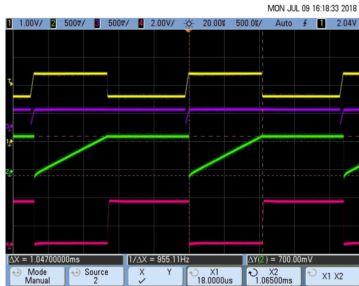
55. Pacemaker Detection Output for 8-mV, 100-μs Pace Pulse
