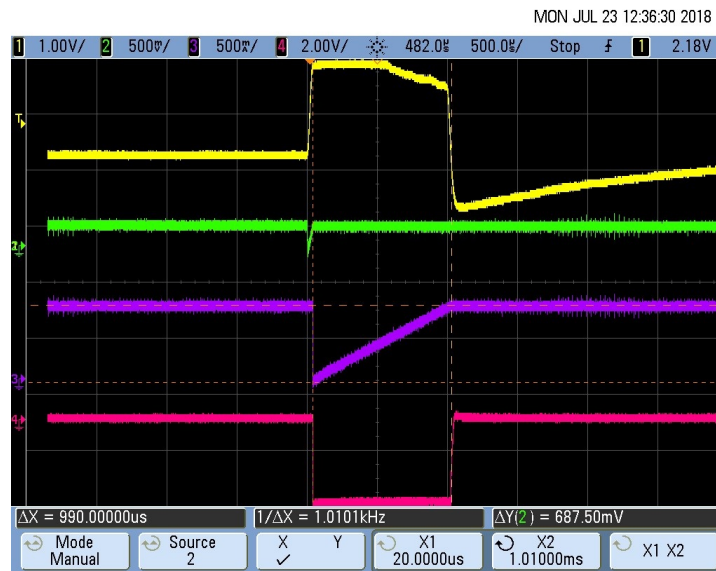
図 71. Pacemaker Detection Output (Pulse Duration T_D ) for 16-mV, 1-ms Pace Pulse
