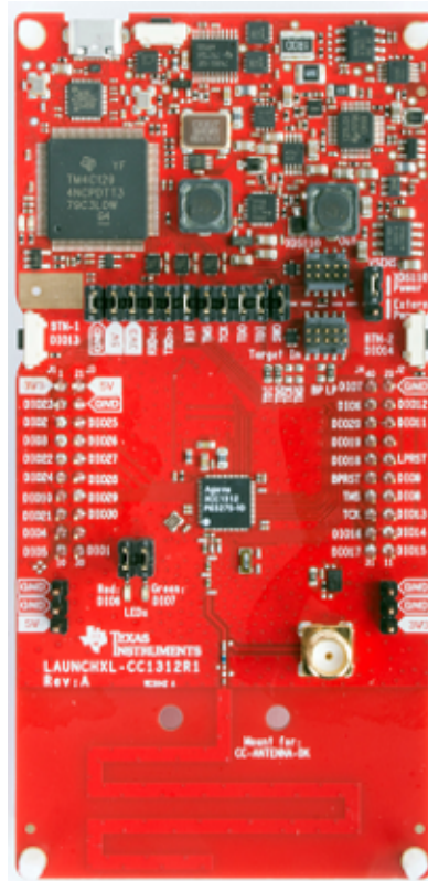
Figure 6. TIDA-010024 Hardware Platform
