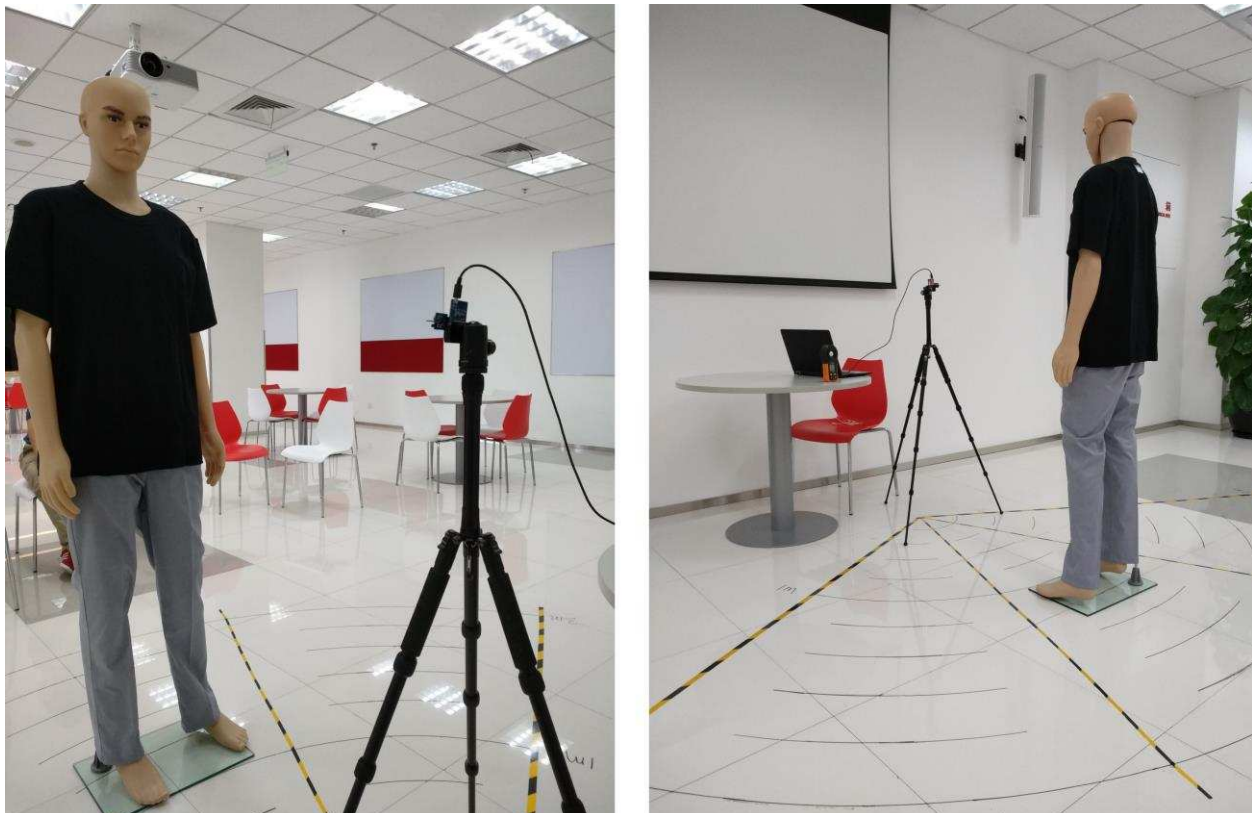
☒ 40. Human Model in Black Color Clothes as Test Target
