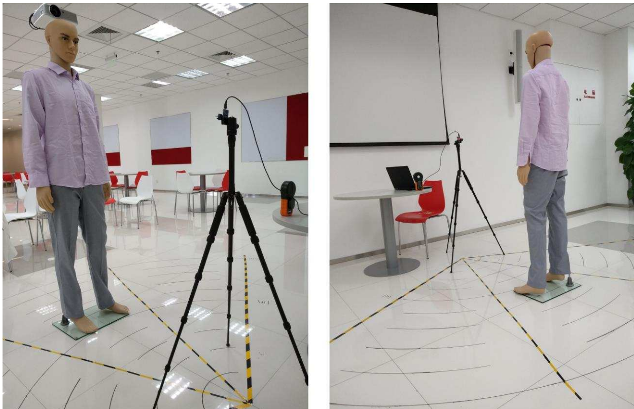
Figure 33. Human Model in Pink Color Clothes as Test Target
