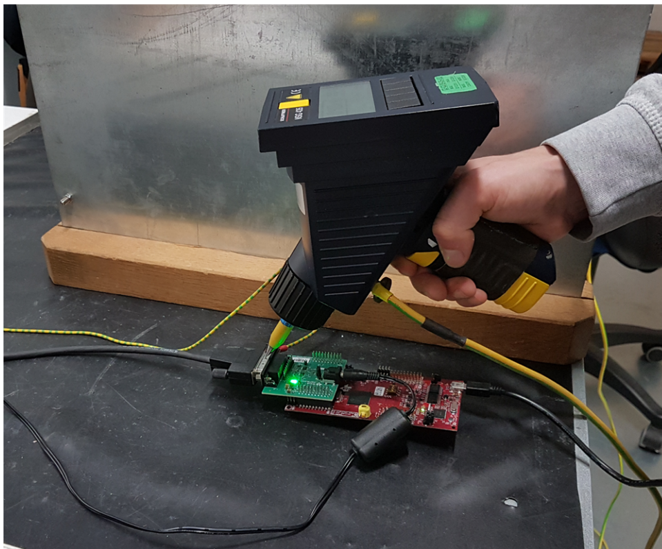
Fig 48. TIDA-010026 Test Setup for ESD Immunity Tests Using Encoder
