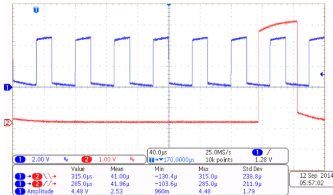
図 44. I2C 100 Kbps: Isolated SCL (Blue) and SDA (Red)
