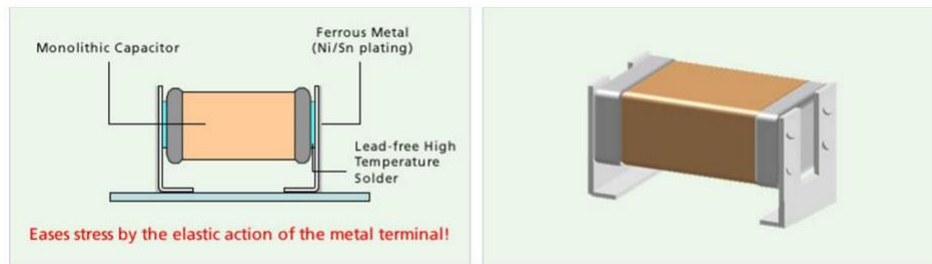
図 12. Standoff Capacitors
