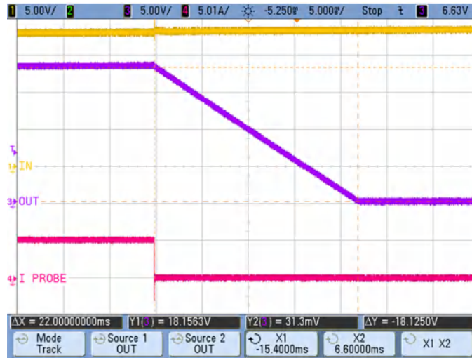
図 3-1. Over-Voltage Protection Cut-Off Mode
