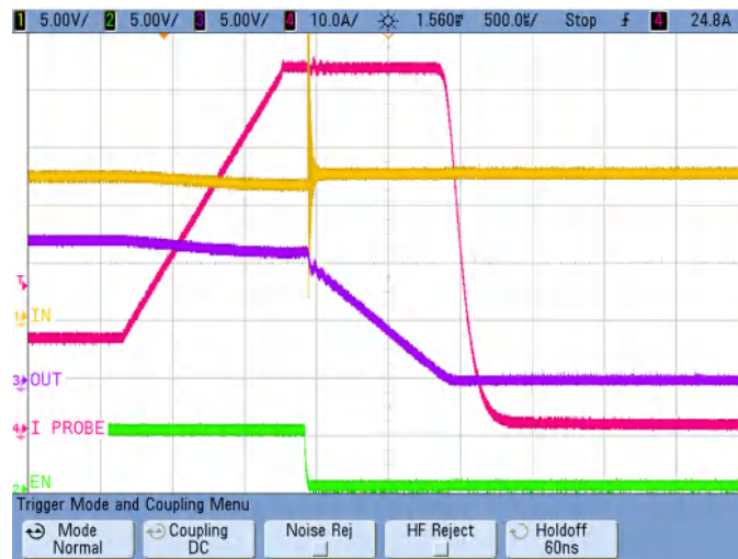
図 3-6. Latch Mode Overcurrent Protection
