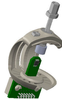
Figure 4. TMAG5170 Orbital Attachment
