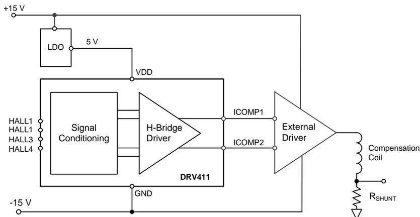
Figure 55. DRV411 Application Example:  $\pm 15$ -V Sensor Modules
