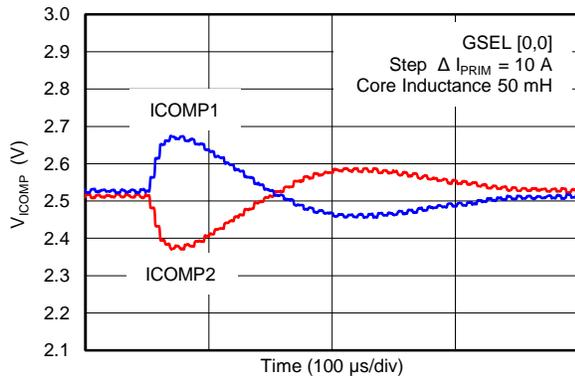
**Figure 49. Settling of ICOMP1 and ICOMP2 (Mode Gain\_1)**
