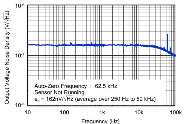
**Figure 36. DIFFERENTIAL AMPLIFIER OUTPUT VOLTAGE NOISE DENSITY**
