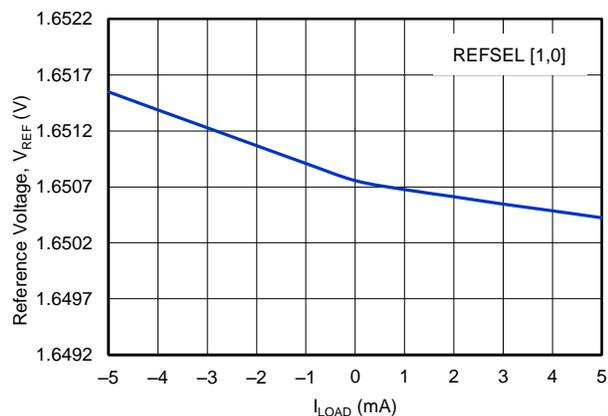
**Figure 41. 1.65-V REFERENCE OUTPUT VOLTAGE vs LOAD CURRENT**
