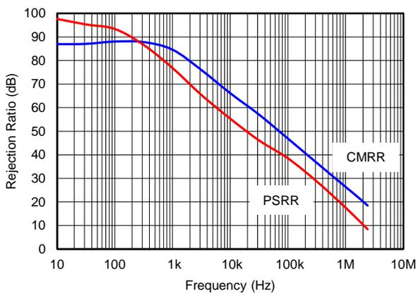
**Figure 17. DIFFERENTIAL AMPLIFIER CMRR AND PSRR vs FREQUENCY**
