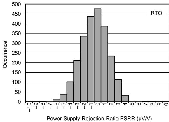
**Figure 19. DIFFERENTIAL AMPLIFIER POWER-SUPPLY REJECTION RATIO HISTOGRAM**
