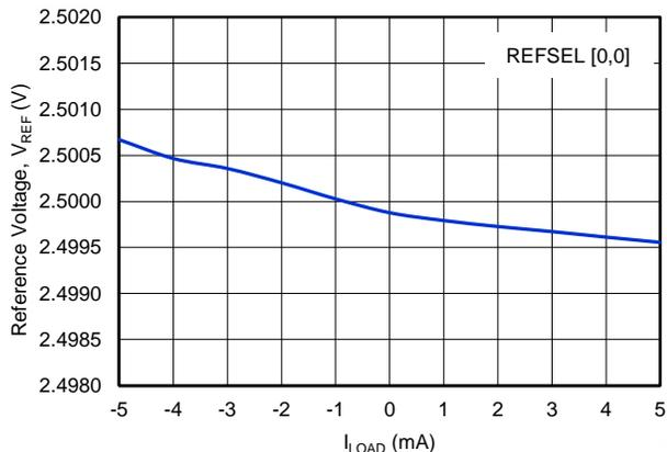
**Figure 37. 2.5-V REFERENCE OUTPUT VOLTAGE vs LOAD CURRENT**
