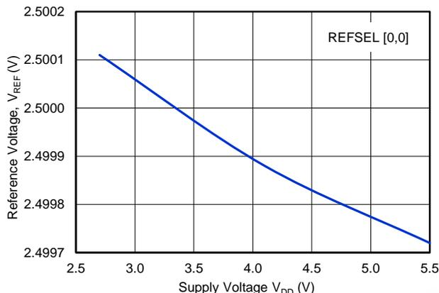
**Figure 40. 2.5-V REFERENCE OUTPUT VOLTAGE vs POWER SUPPLY**
