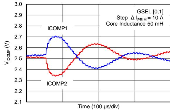
**Figure 50. Settling of ICOMP1 and ICOMP2 (Mode Gain\_2)**
