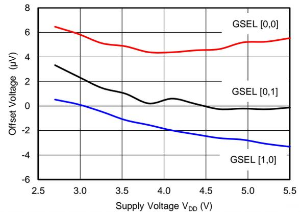
**Figure 10. FRONT-END OFFSET VOLTAGE vs POWER SUPPLY**
