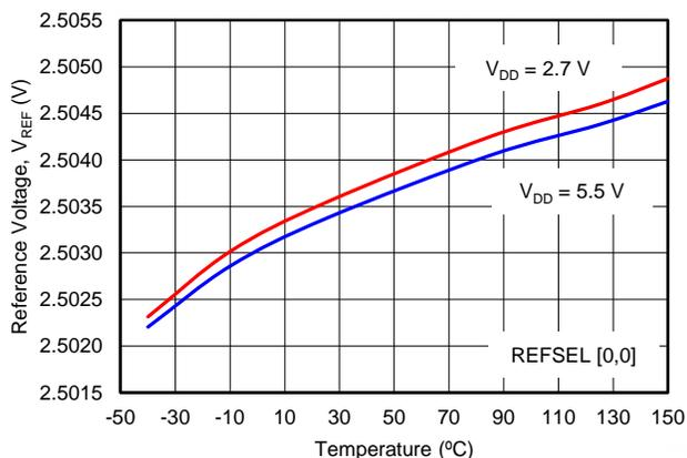
**Figure 39. 2.5-V REFERENCE OUTPUT VOLTAGE vs TEMPERATURE**
