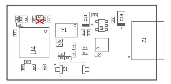
Figure 4-10. PCB Bottom-Layer Assembly Drawing
