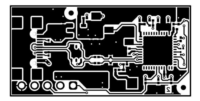
Figure 4-8. PCB Bottom Layer
