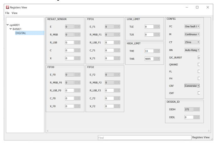
Figure 3-21. Registers View Example for OPT4xxx Devices
