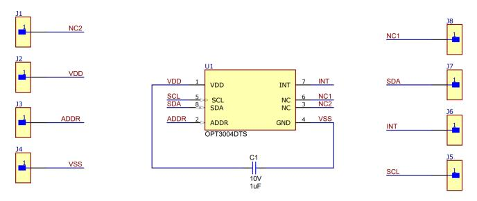
Figure 4-1. OPT3004 Coupon Board Schematic
