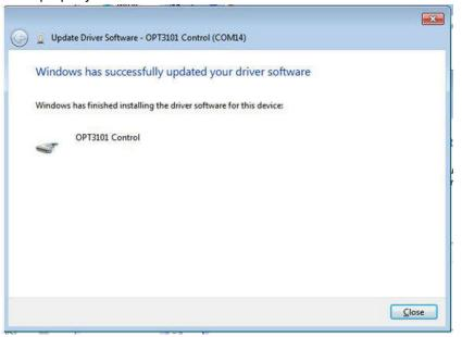
14. Now repeat this process (steps 1 to 13) for the second *USB Serial Device*. All steps are the same except for step 2 and step 11. In step 2, make sure to right-click the second *USB Serial Device*. Likewise, on step 11 make sure to select the second *USB Serial Device* when installing the driver as the following figure shows.
