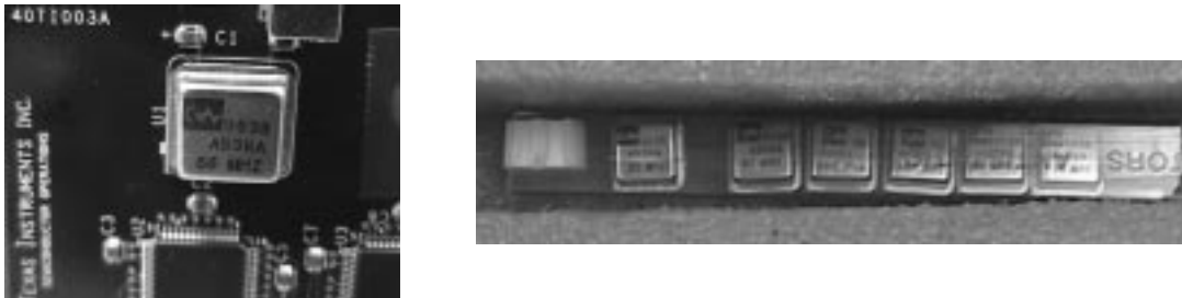
Figure 2–11. Clock Crystal on Card (Left) and Stored in Tube (Right)
