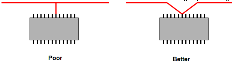
Figure 2-5. Avoid Right-Angle Traces
