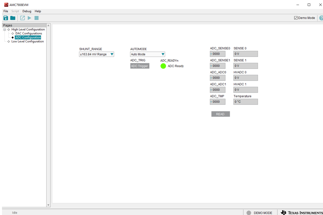
Figure 3-8. ADC Control Tab of the High Level Configuration Page
