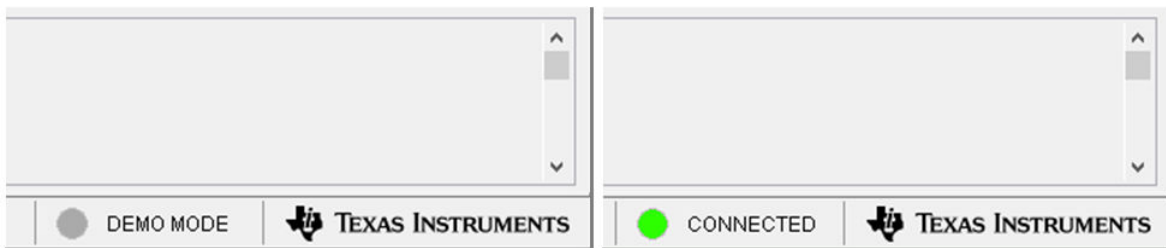
Figure 3-5. FTDI Digital Controller Connection Status
