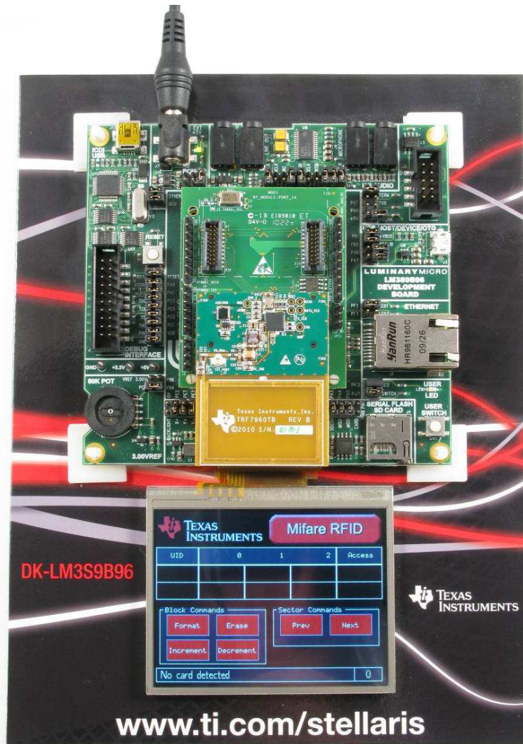
Figure 11. DK-LM3S9B96-EM2-TRF7960R Development Platform
