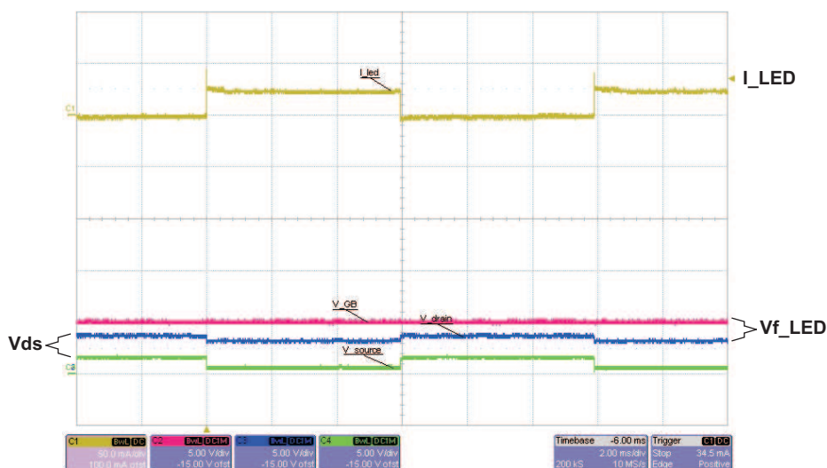
Figure 2. One LED With 5-V LED Supply Voltage, LED Current (Yellow), V_{GB} (Pink), Voltage on MOSFET's Drain (Blue), and Voltage on MOSFET's Source, or on OUTx Pin (Green).
