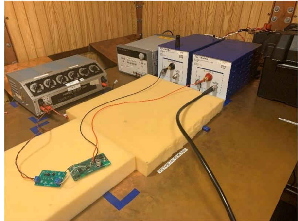
Figure 1-2. Test Setup for Conducted Emission Loaded Measurement
