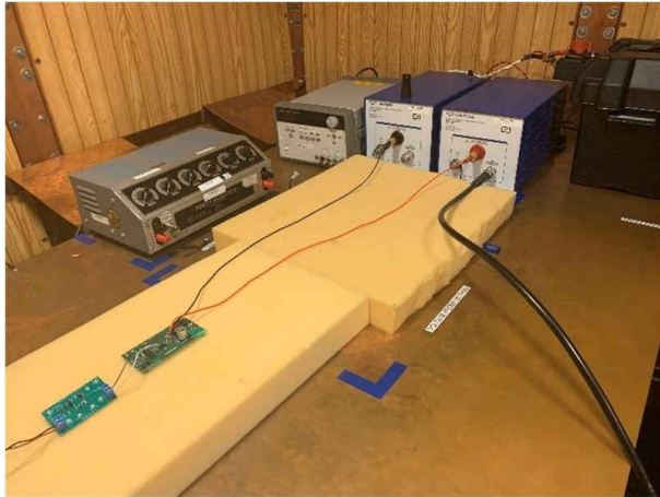
Figure 1-1. Test Setup for Conducted Emission Noise Floor Measurement
