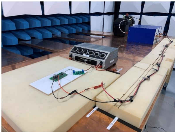
Figure 1-3. Test Setup for Radiated Emission Measurement
