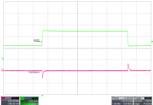
Figure 5-18. Load Transient, CH2, V_{IN} = 13.5\text{ V} , I_{OUT2} = 2.5\text{ A} to 5\text{ A} at 1\text{ A}/\mu\text{s}
