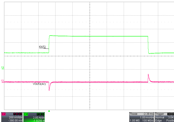
Figure 5-17. Load Transient, CH2, V_{IN} = 6\text{ V} , I_{OUT2} = 2.5\text{ A} to 5\text{ A} at 1\text{ A}/\mu\text{s}
