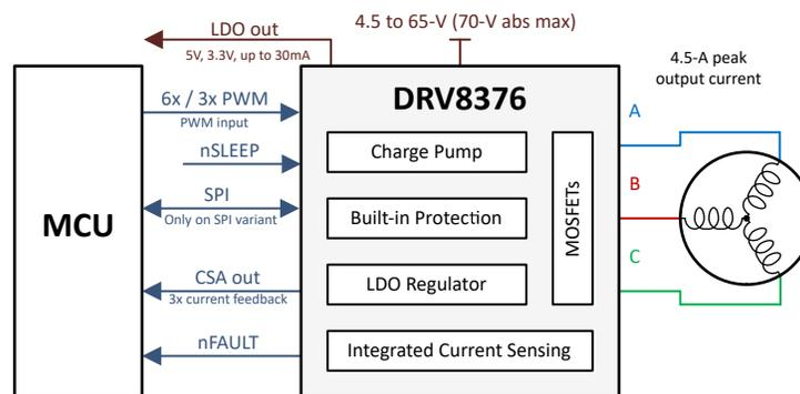
**Figure 1-1. Simplified Schematic**
