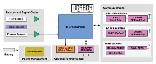
Figure 2. A TI-enabled smart flow meter solution featuring various connectivity options
