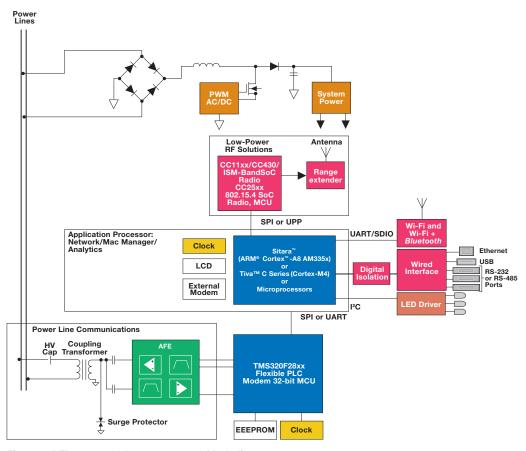
Figure 4. A TI-connected data concentrator block diagram
