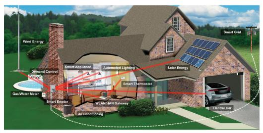
Figure 5. Smart grid connectivity enabling smart home services
