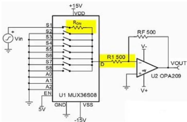
**Effective Gain (AG) =  $-\frac{R_F}{R_1 + R_{ON}}$**
