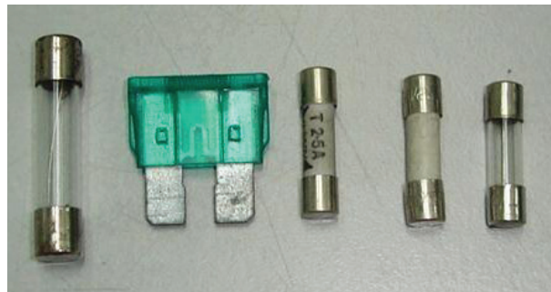
Figure 2. Different styles and sizes of simple fuses.
