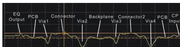
Figure 2. Example TDR Plot of Impedance Across the Signal Path (See Figure 1 for discontinuity locations)
