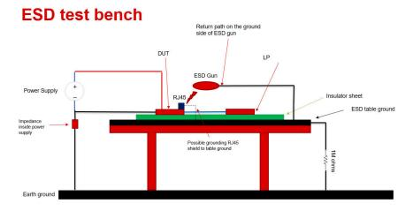
Figure 4-3. ESD Test Setup
