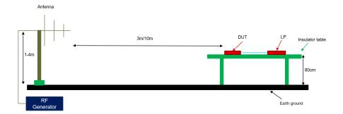
Figure 3-3. RE Test Setup
