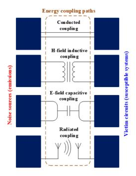
Figure 2-2. Noise Coupling Path
