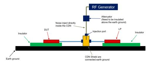
Figure 4-11. CI Test Setup
