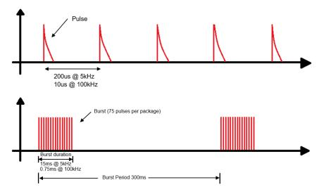
Figure 4-6. EFT Test Waveform
