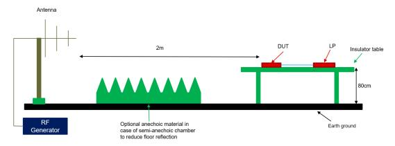
Figure 4-5. RI test setup
