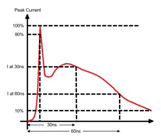
Figure 4-2. ESD test waveform
