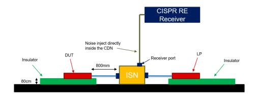
Figure 3-4. CE Test Setup
