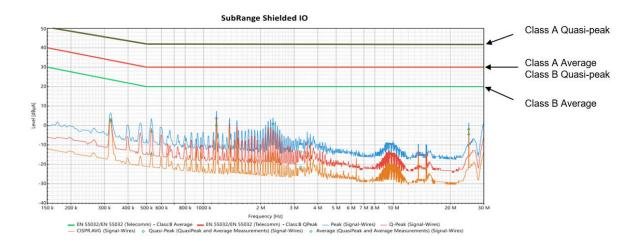
Figure 3-2. CISPR 32 CE Passing Criteria
