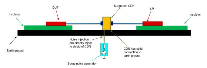
Figure 4-10. Surge Test Setup on Noise Injection on CDN
