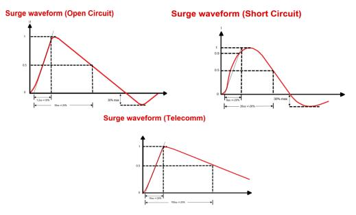
Figure 4-8. Surge Test Waveform
