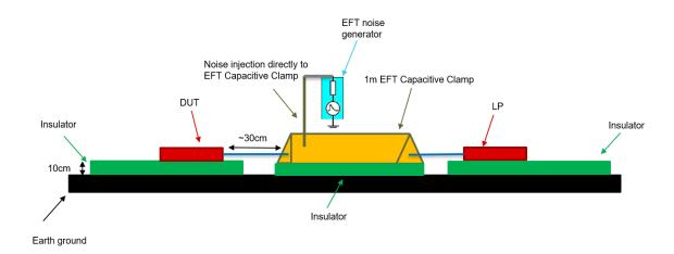
Figure 4-7. EFT Test Setup
