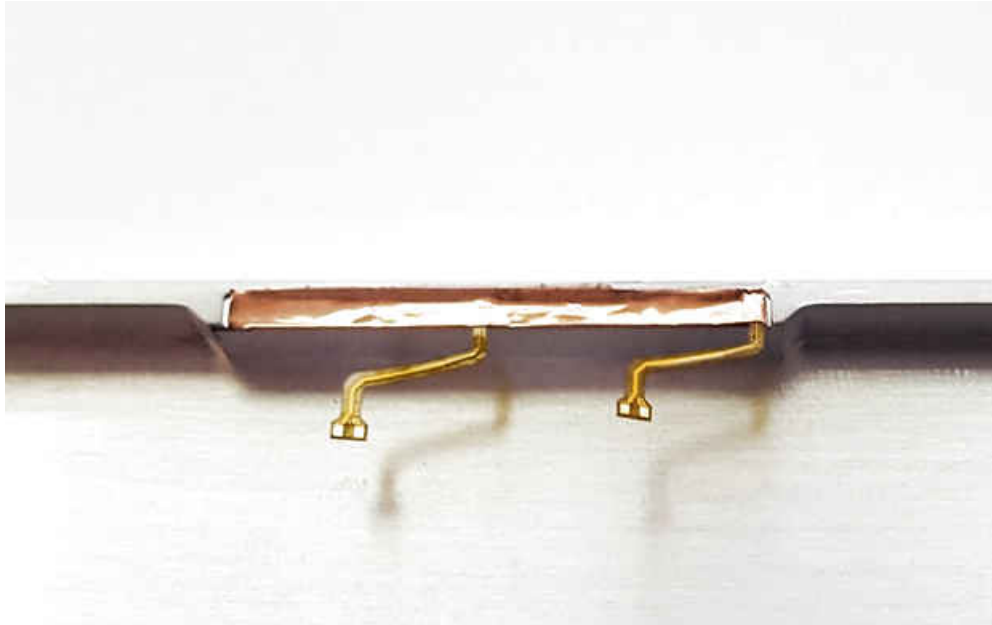
Figure 1-13. Copper Foil Shielded “Faraday Box”
