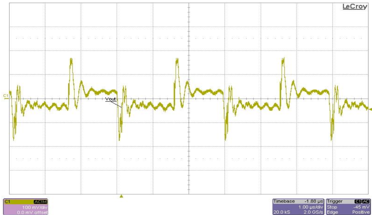
8Vin, 1A load. Ch1 measures output ripple.
