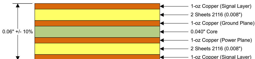
Figure 5. Typical Four-Layer PCB Stack with Routing Assignments
