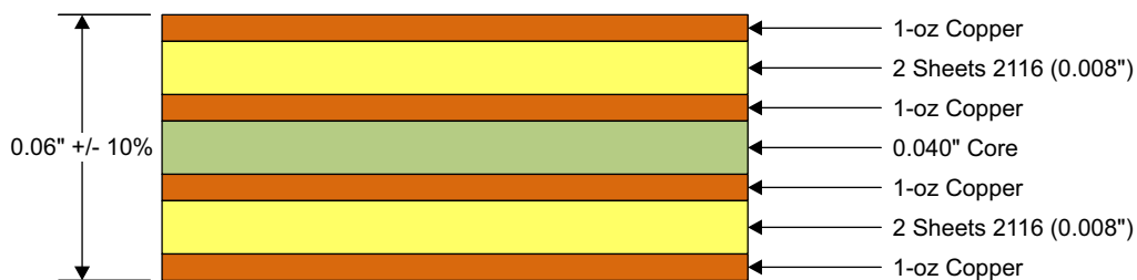
Typical 4 Layer PCB Stack
