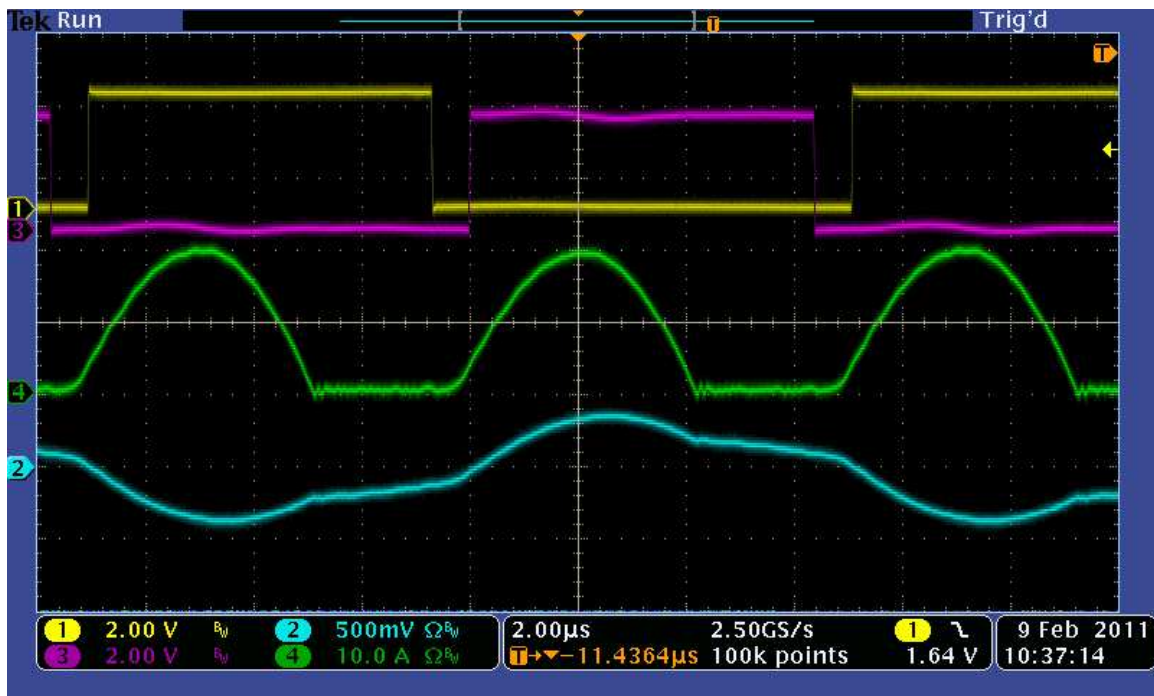
Figure 23. Operational Current Waveforms (Yellow – HB HS PWM, Purple – HB LS PWM, Green – Combined SR Currents, Blue – Tank Current)
