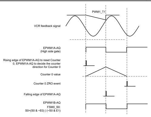
Figure 3-3. CLB Logic for Primary Side PWM
