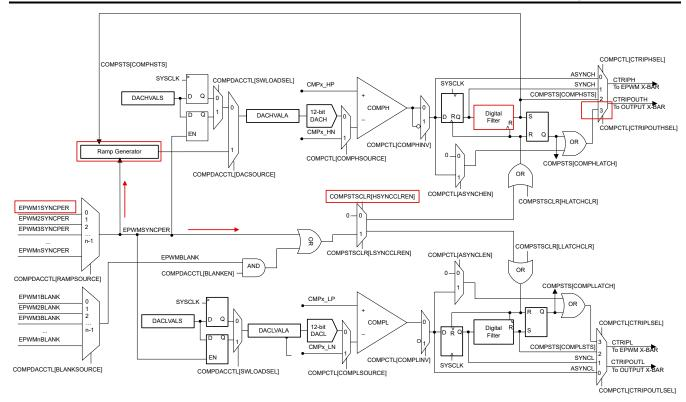
Figure 3-1. CMPSS Block Diagram
