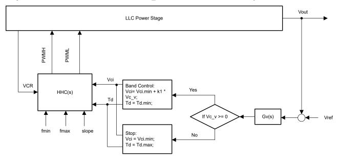
Figure 4-3. Control Algorithm During the Normal Operation
