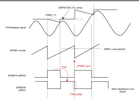
Figure 2-2. HHC LLC Control Architecture
