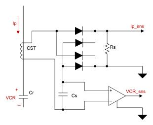
Figure 5-1. Simplified VCR Sensing Circuits
