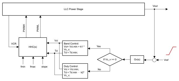
Figure 4-2. Control Algorithm During the Soft Start
