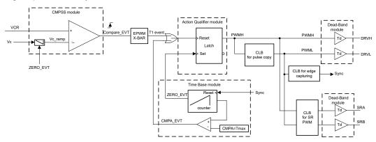
Figure 2-3. Block Diagram of the System Control Logic Within C2000
