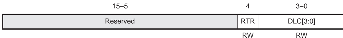
Figure 10–7. Message Control Field (MSGCTRLn)
