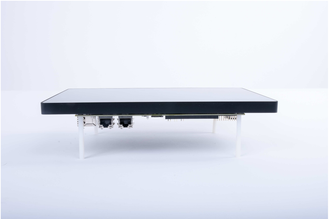
Figure 4. AM571x IDK EVM with LCD Display Assembly Attached
