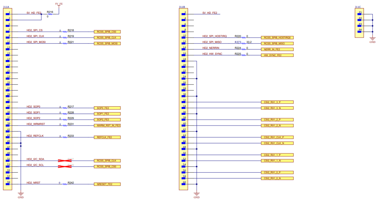
Figure 2-26. High Density FE Connector-2 Schematic
