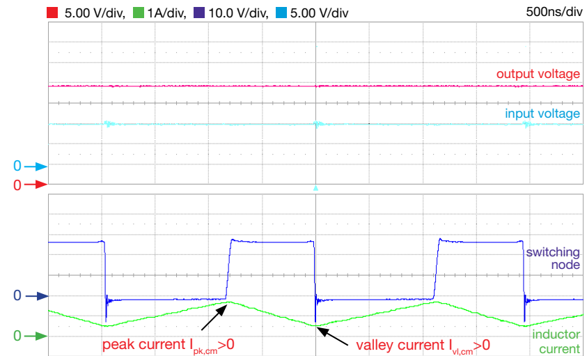
Figure 10. Boost converter operation with SOM setup at high load ( I_{out} > I_{dcm} ): V_{in}=10V , I_{out}=0.4A , nominal f_s=500kHz (real f_s=513kHz ), L=10\mu H
