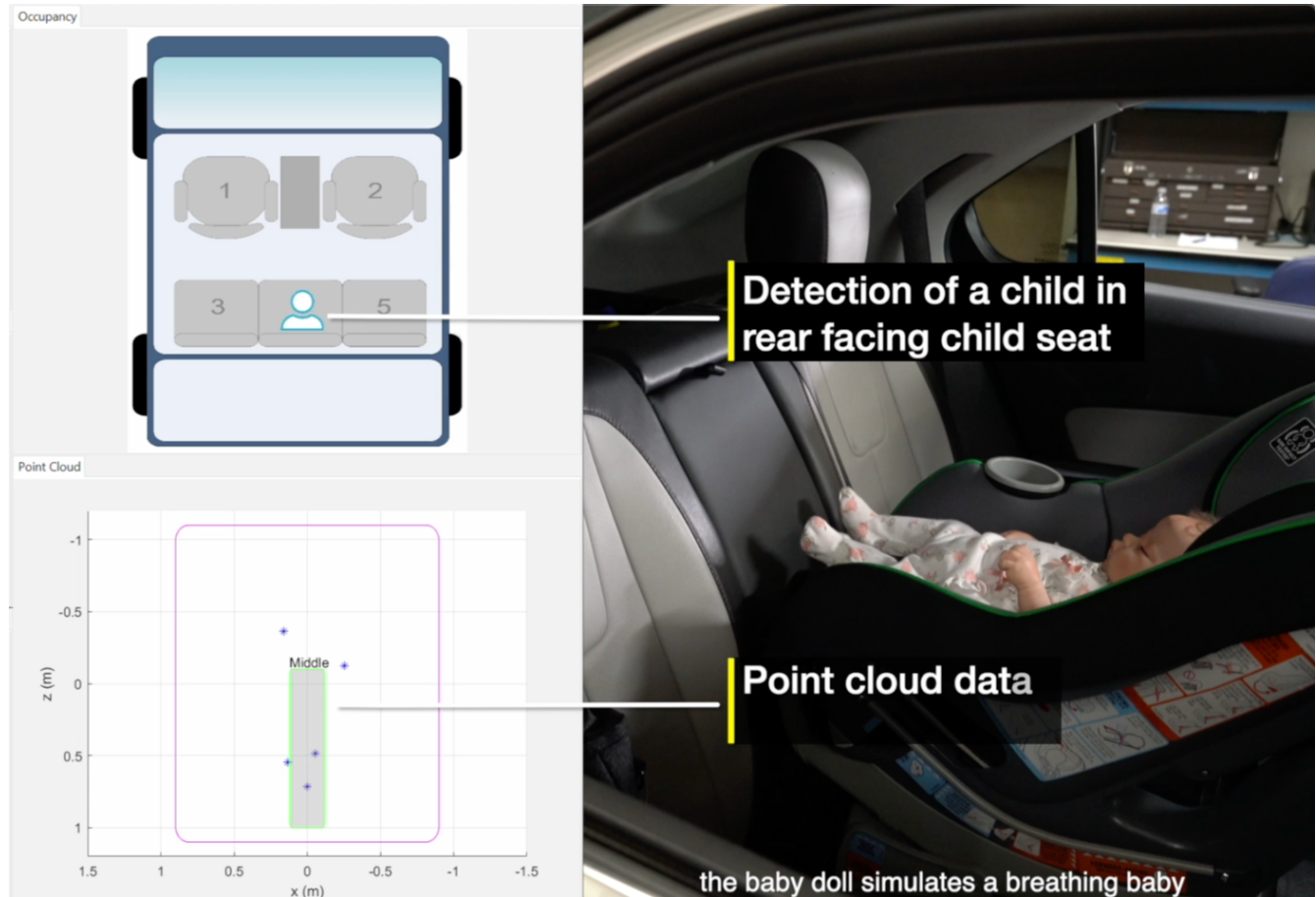
Figure 5. Detection of a child (a baby doll simulating a breathing child) in the rear seat of a vehicle ( video )
