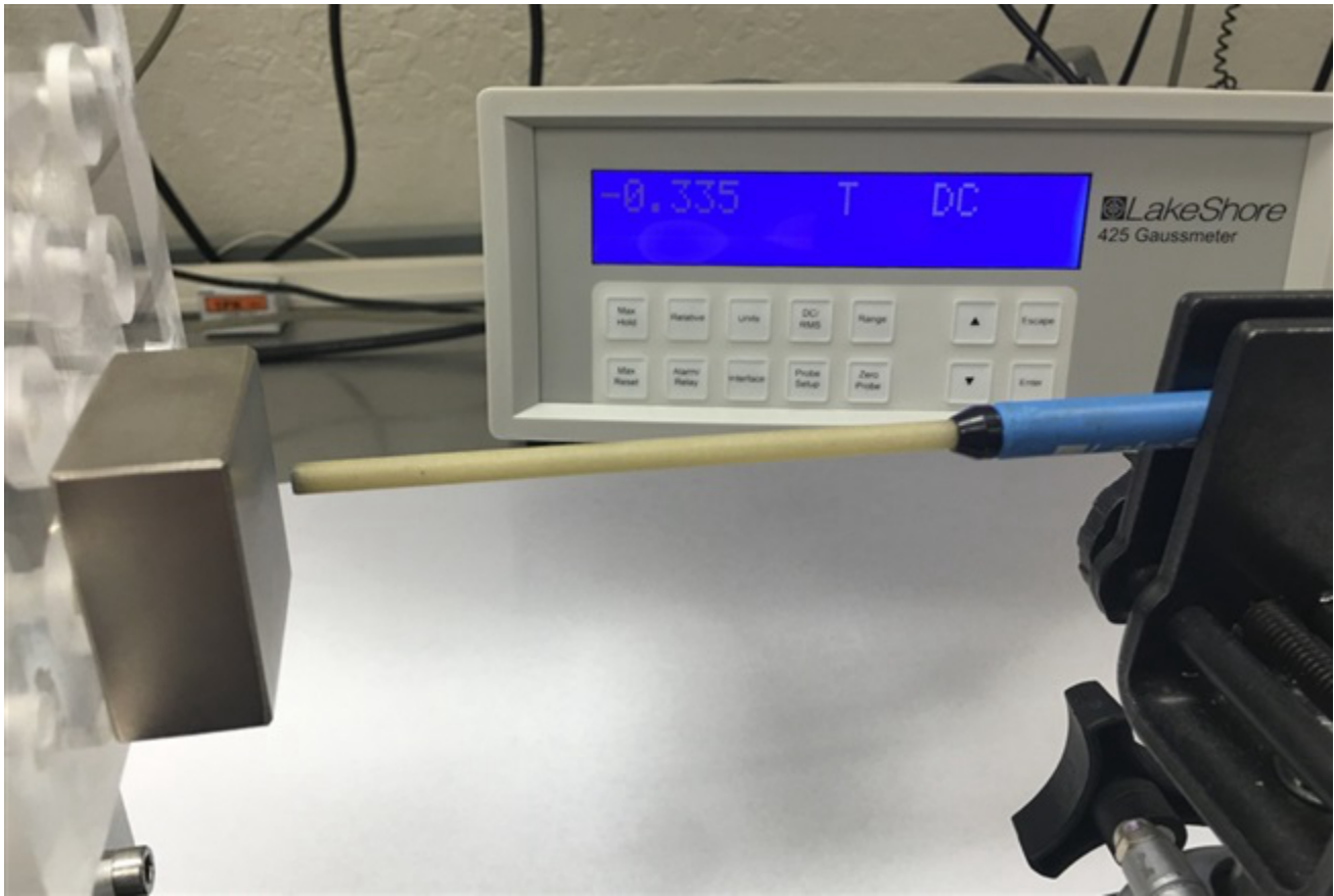
Figure 2. The Gauss Meter Shows That the Magnet Has a Magnetic Field Strength of 335mT at a 3mm Distance
