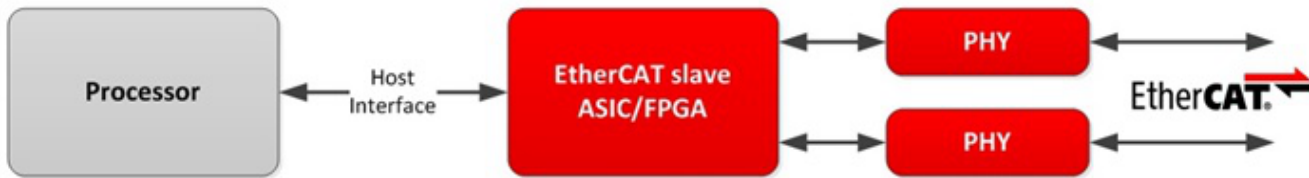
Figure 2. EtherCAT Slave with an ASIC/FPGA and External Processor
