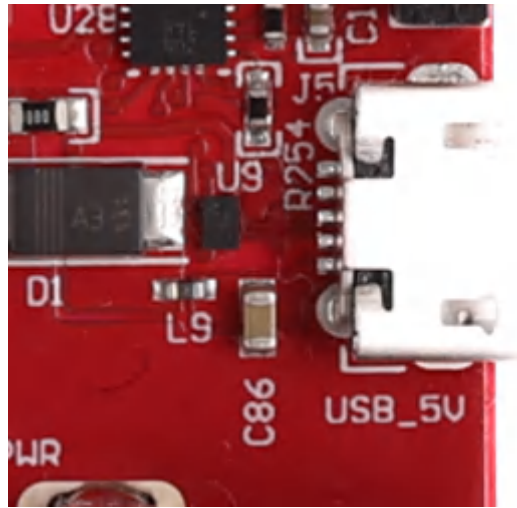
Figure 2-13. USB Connector (J5)
