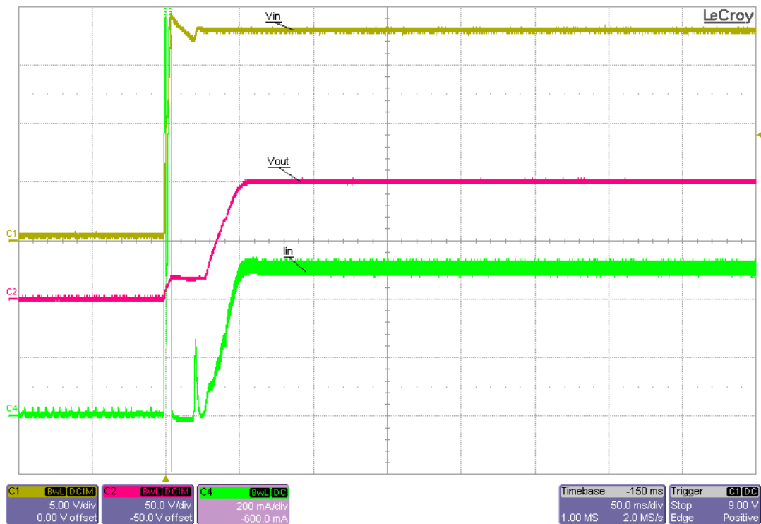
Figure 20. Startup Into 85 mA Resistive Load, 18-V Input, 100-V Output
