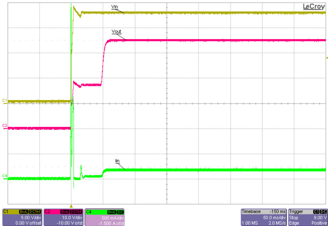
Figure 19. Startup Into 85 mA Resistive Load, 18-V Input, 35-V Output
