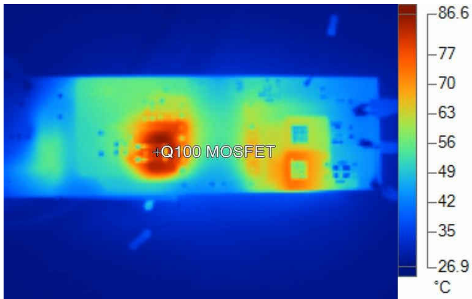
Figure 2-4. 110-VAC Input Top Thermal Image
