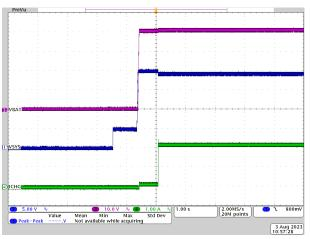
Figure 3-4. 20Vsys to 10S BAT = 40V Charge Mode
