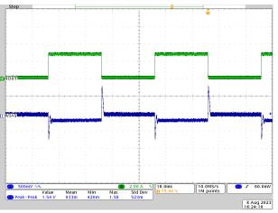
Figure 3-18. OTG Mode, 15V, 10% to 100% Load Dynamic
