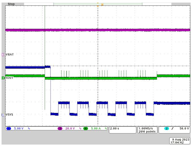
Figure 3-32. Short-Circuit Test at 20V
