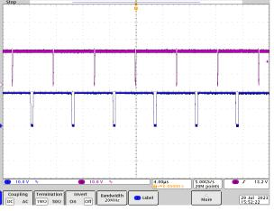
Blue: buck leg switching point, Purple: boost leg switching point Figure 3-22. Buck-Boost Mode
