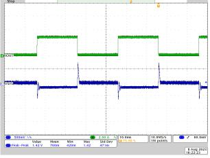
Figure 3-19. OTG Mode, 9V, 10% to 100% Load Dynamic
