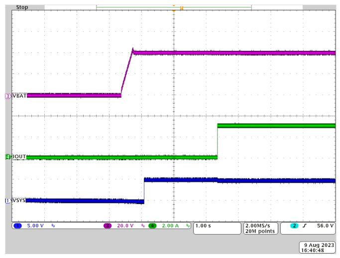
Figure 3-5. 40Vbat, Start-Up at 5V Input Source
