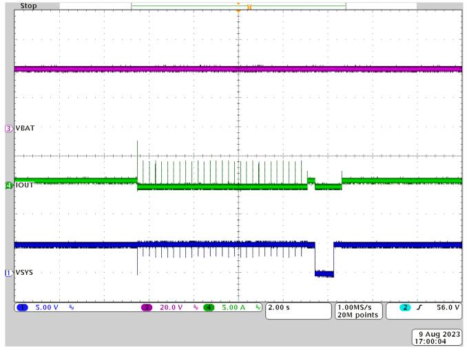
Figure 3-29. Short-Circuit Test at 5V
