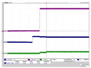
Figure 3-1. 5Vsys to 10S BAT = 40V Charge Mode
