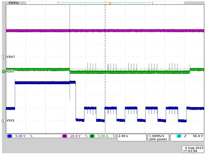
Figure 3-31. Short-Circuit Test at 15V
