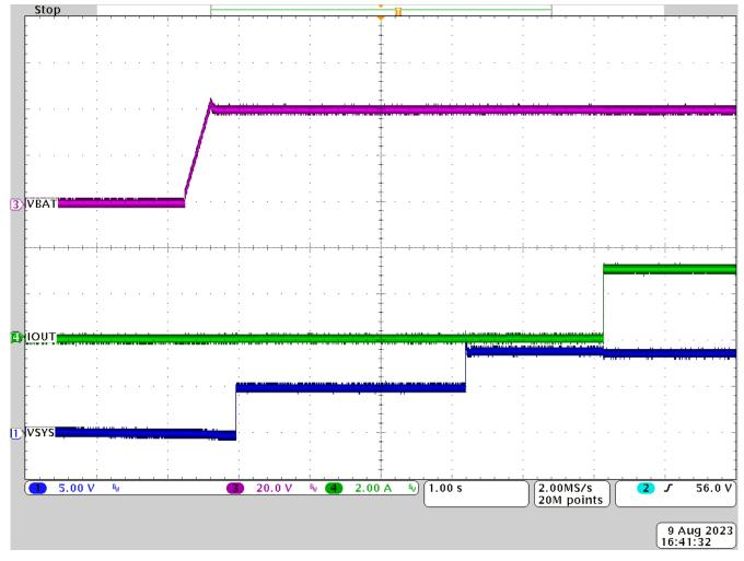
Figure 3-6. OTG, 40Vbat, Start-Up at 9V Input Source
