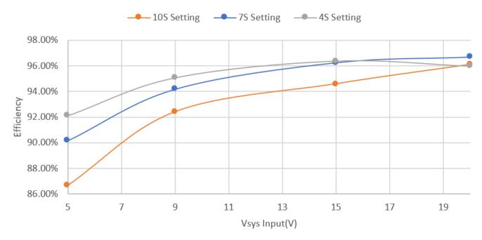
Figure 2-1. Charge Mode Efficiency Across Vsys and Vbat
