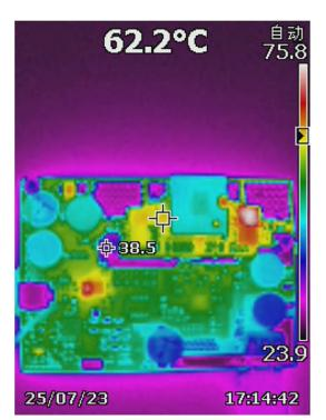
Figure 2-6. OTG Mode From Vbat = 42V to 20V at 5A
