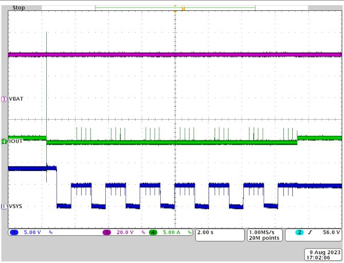
Figure 3-30. Short-Circuit Test at 9V
