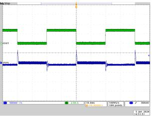
Figure 3-20. OTG Mode, 5V, 10% to 100% Load Dynamic
