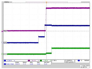
Figure 3-3. 15Vsys to 10S BAT = 40V Charge Mode
