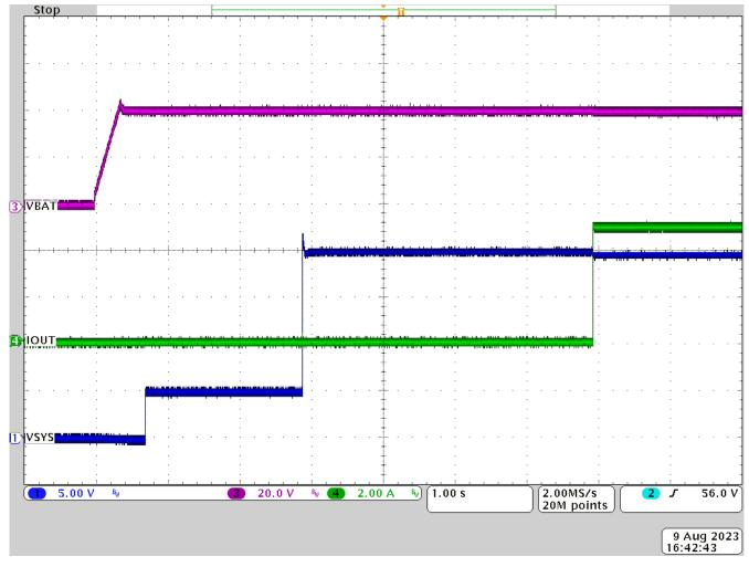
Figure 3-8. OTG, 40Vbat, Start-Up at 20V Input Source
