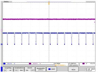
Blue: buck leg switching point, Purple: boost leg switching point Figure 3-21. Buck Mode
