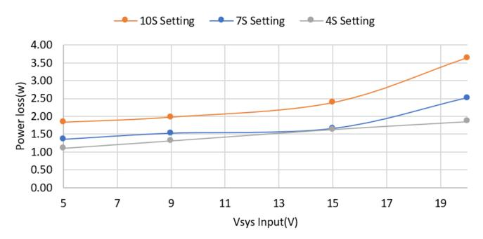
Figure 2-2. Power Loss vs Vsys and Vbat
