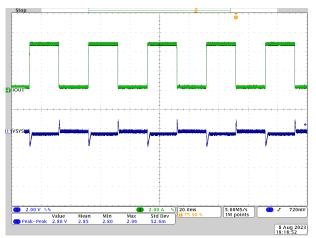
Figure 3-17. OTG Mode, 20V, 10% to 100% Load Dynamic
