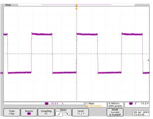
Figure 3-24. Switching Leg Waveform at Vsys = 20V, Vbat = 40V Full-Load Charging Mode, f<sub>SW</sub> = 300kHz
