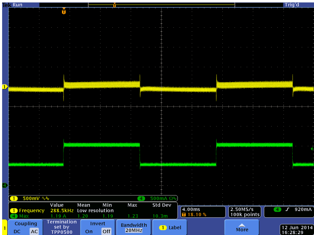
Fig 4 Transient Response, Vin=48V Io=50%~100%~50%
