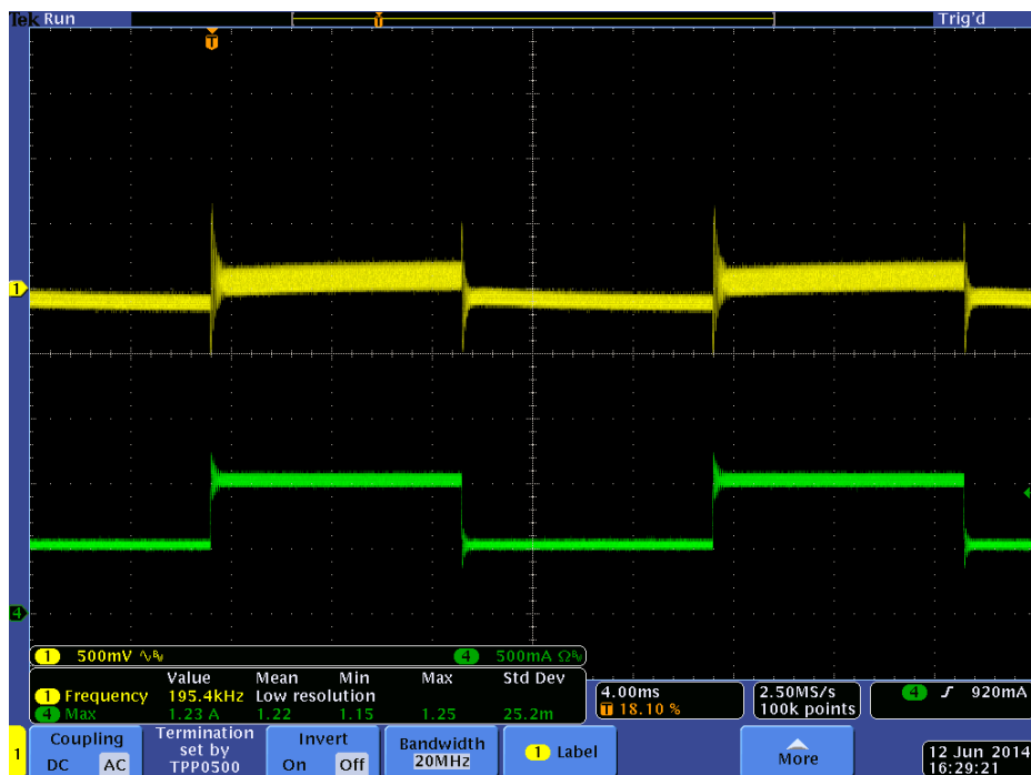
Fig 5 Transient Response, Vin=57V Io=50%~100%~50%
