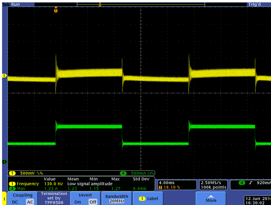
Fig3 Transient Response, Vin=33V Io=50%~100%~50%
