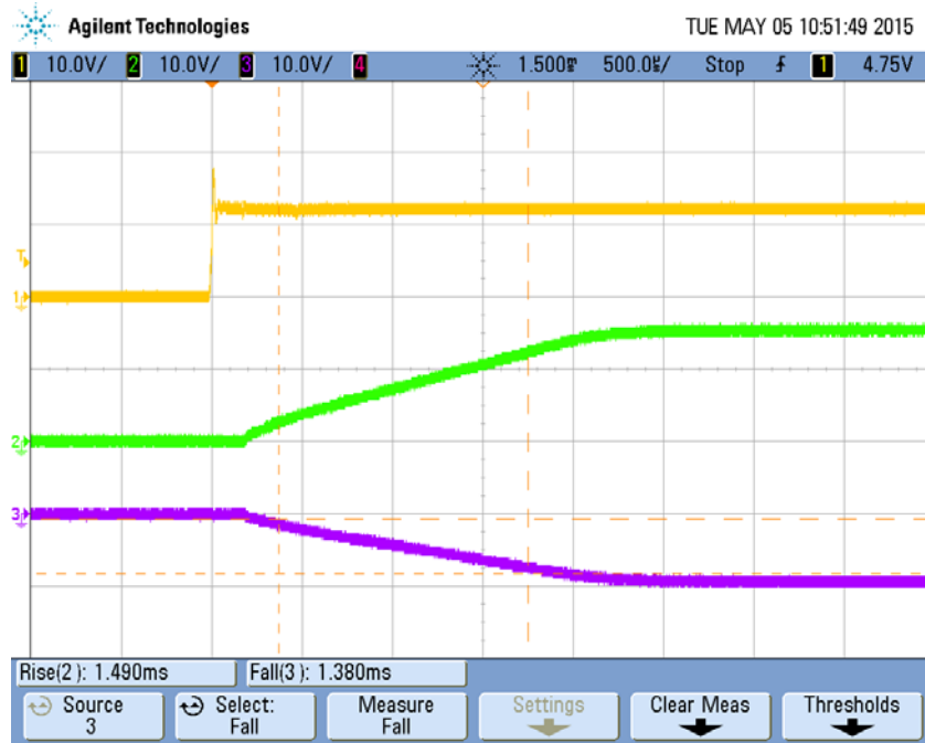
Figure 15 Power up into no load at 12V input
