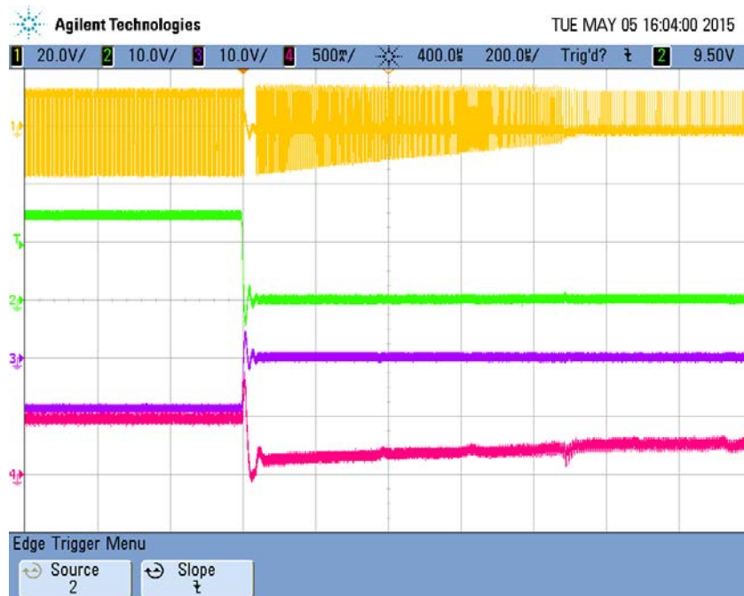
Figure 25 From full load operation to short circuit at 12V input
