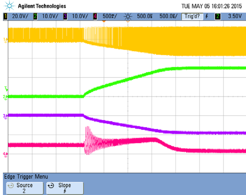
Figure 26 Short circuit removed into full load operation at 12V input
