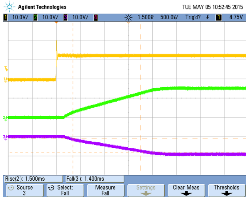
Figure 16 Power up into full load at 12V input
