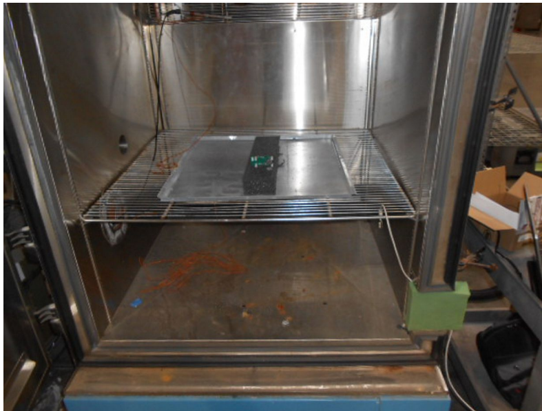
Figure 18. Wireless PIR Motion Detector Temperature and Humidity Test Setup
