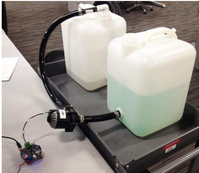
Figure 59. Simple Water Pump Hardware
