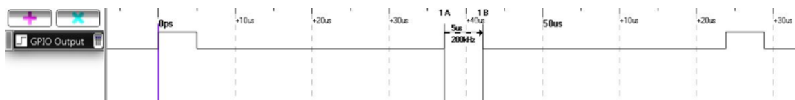
Figure 17. Time to Process a Packet by RxPktTransfer_ESL Function
