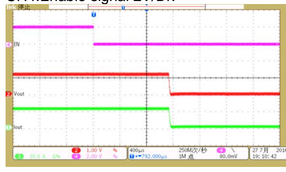
Full load CH2: Output voltage 1V/Div CH3: Load Current 10A/Div CH4: Enable signal 2V/Div
